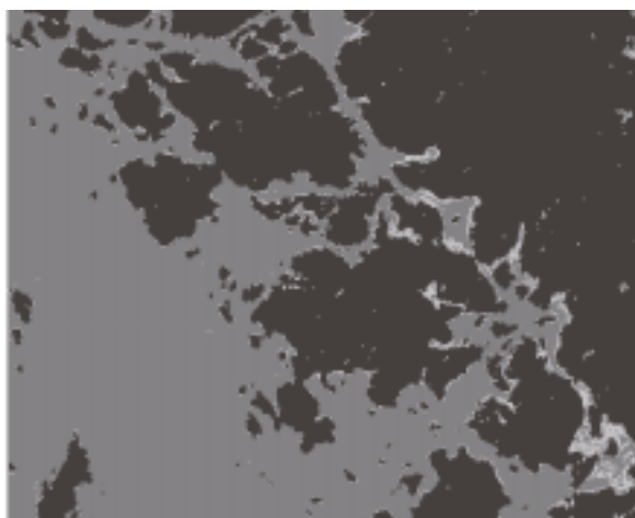
Figure 3.7 Outcome of supervised classification, refined method. The view is from Råssö and Galtöleran. Light areas are algae, grey areas are water and dark areas are land.
