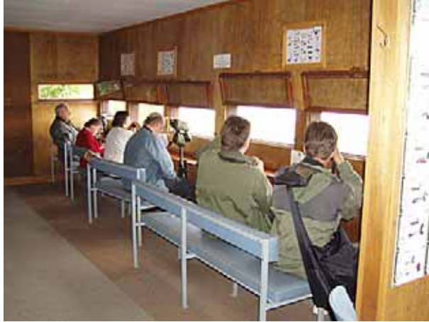
A hide dimensioned for a large number of visitors. Equipped with comfortable movable benches, which also allows visitors bound to wheelchairs to use the view openings.
