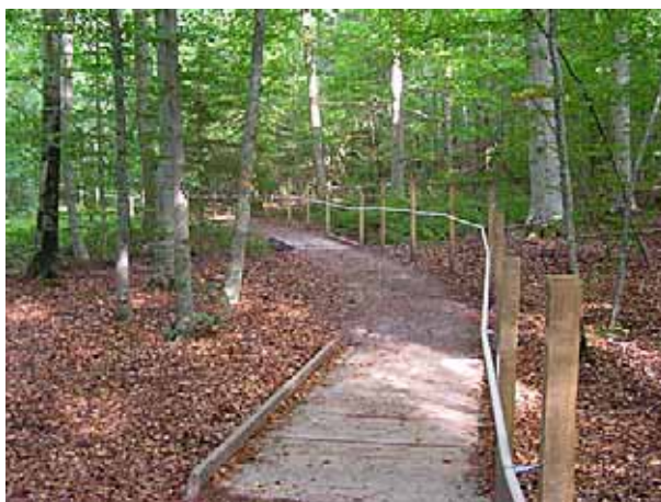
With a rope to follow with the hand a blind person can walk this trail independent.
