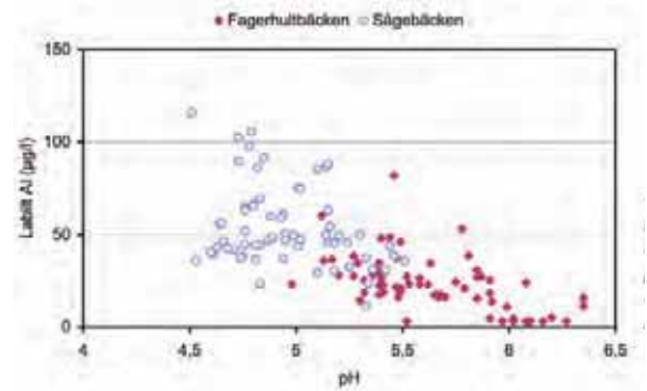
Diagram 15. Labilt aluminium ug/l avsatt mot pH (Abrahamsson 2007 (1))
