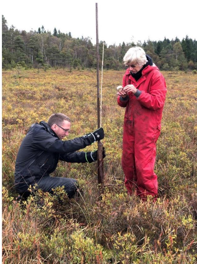
Figure 4. Measuring the extension rod and marking depth for the second drive.
