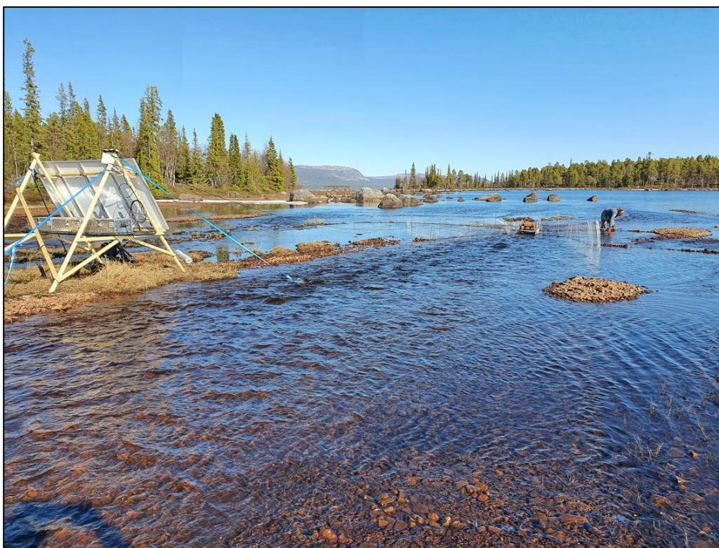
Figure 34. The fish counter, Simsonar FC, reinstalled on 29 May because the counter was moved due to high water pressure. Guide nets were also installed to guide fish during downstream migration. Battery storage as well as PC and router for internet connection were stored in the light metal boxes on the back of the solar panels. Photo: County Administrative Board in Norrbotten.
