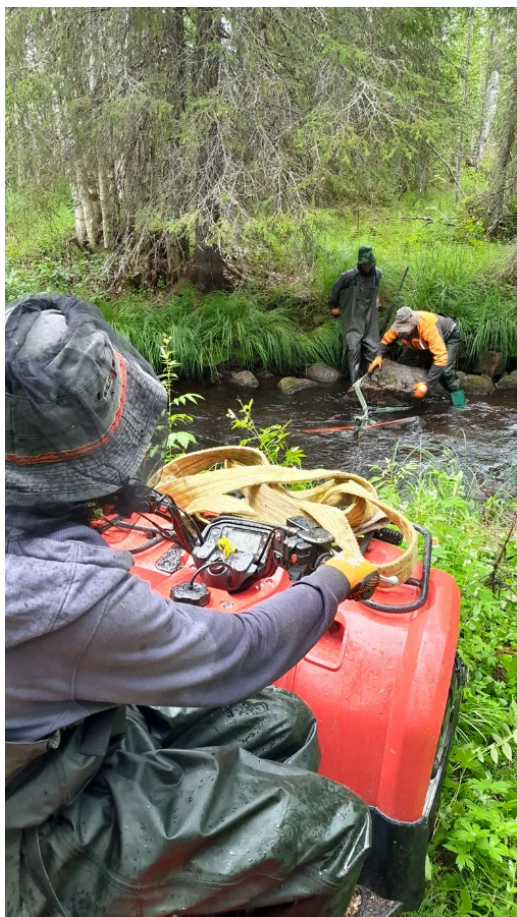
Figure 60. ATV winch can be used for moving bigger boulders. Photo: Markku Vierelä, Metsähallitus
