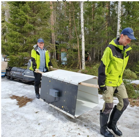
Figure 31. The fish counter consists of a photo tunnel (the white box) with a mounted camera (the gray box on the black side wall) and two lights tubes on the inside. Photo County Administrative Board in Norrbotten.
