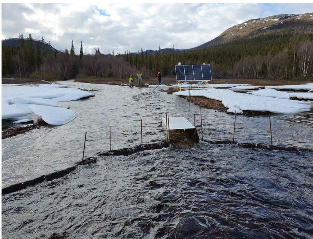
Figure 33. Installed fish counter Simsonar FC with entry fence guiding fish into the fishcounter in Tsåkesjokk and solar panels for recharging batteries on May 26, 2021. Photo: Norrbotten County Board.
