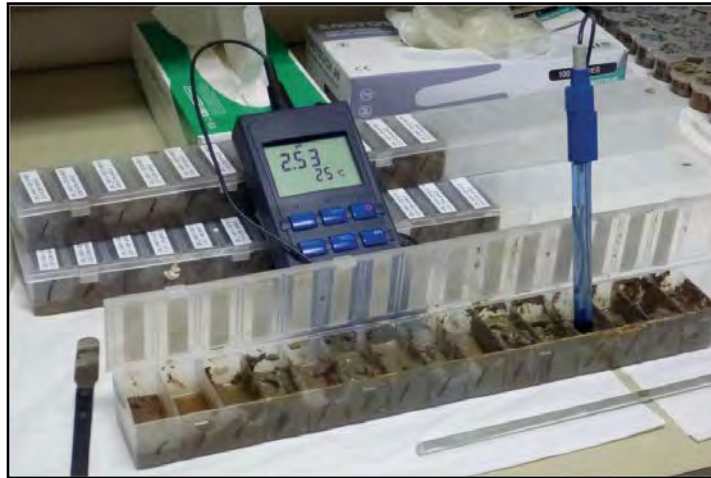
Figure 1. Incubation of soil samples in a chip tray. Photograph: Pentti Kouri, GTK.
