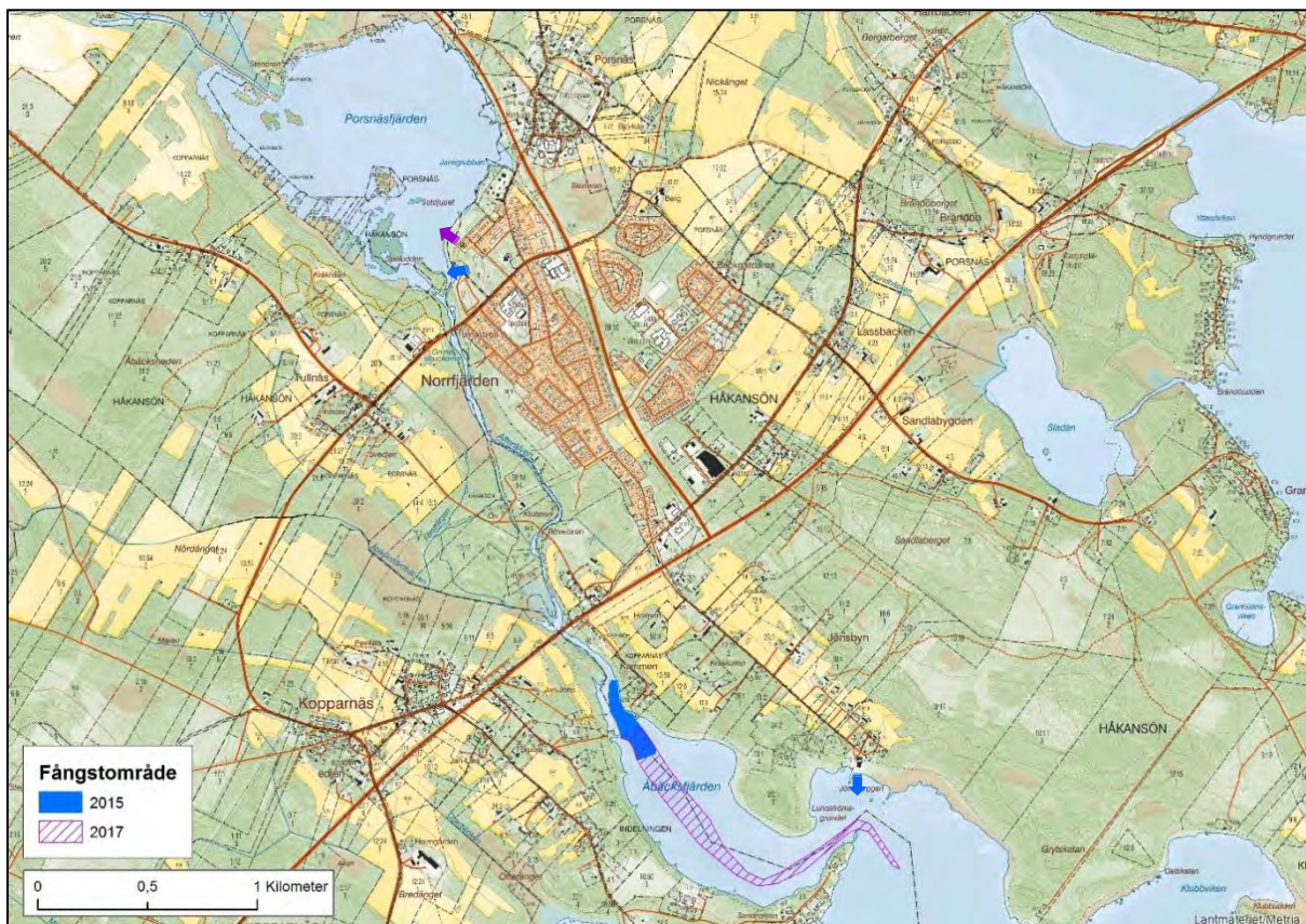
Figure 2.5. Map of the Alterälven river and the positioning of the telemetry study in 2015 and 2017. Blue arrows show the positions of fixed receivers and the direction of antennae in 2015 and 2017. The purple arrow shows the position and direction of the extra antenna used during the 2017 study to increase resolution at the modified migration barrier.
