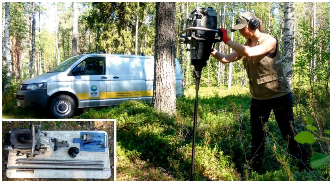
Figure 7. Sampling equipment used for type profiles. The soil sampler is 32 mm in diameter and takes a core that is up to 1 m long. An extension probe is used to take samples at depth. The sampler is hammered into the ground using an Atlas Copco Cobra breaker. Photograph: Krister Dalhem, GTK.
