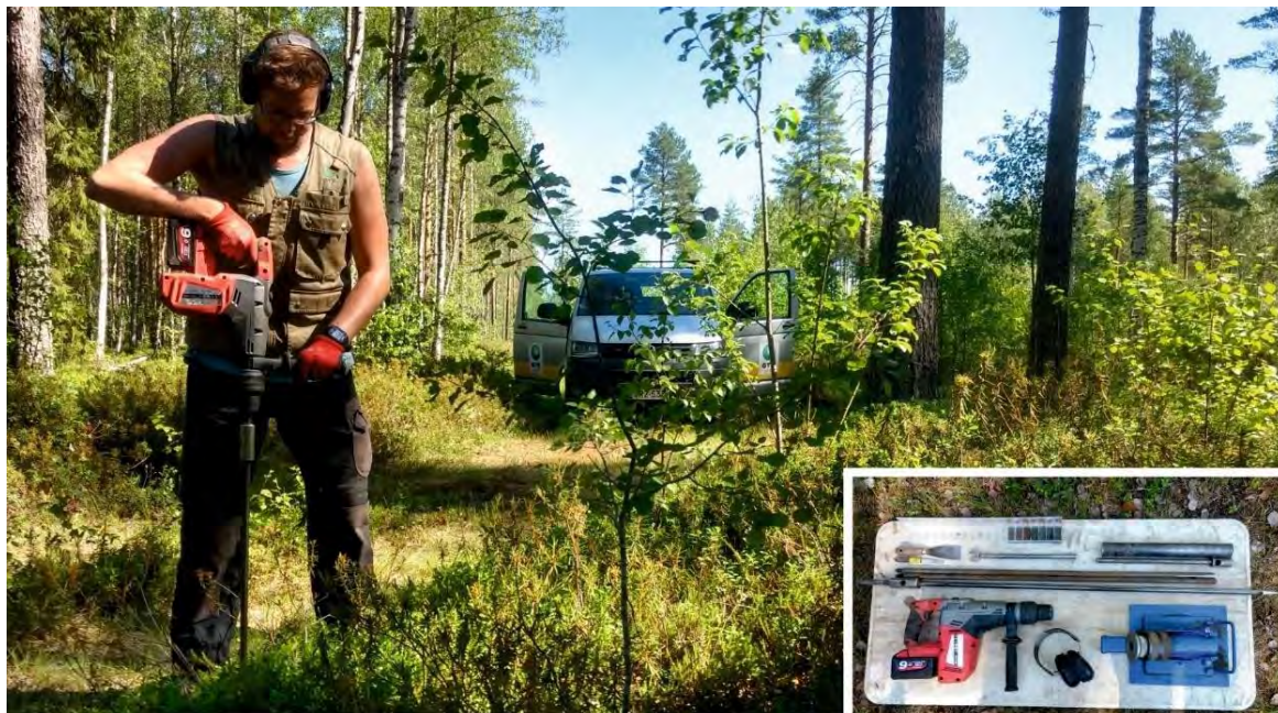
Figure 6. Sampling equipment used for rapid probing. The soil sampler is 18 mm in diameter and takes a core that is up to 1 m long. An extension probe is used to take samples at depth. A hammer drill is used to insert the sampler into the ground. Photograph: Moa Sunabacka, GTK.
