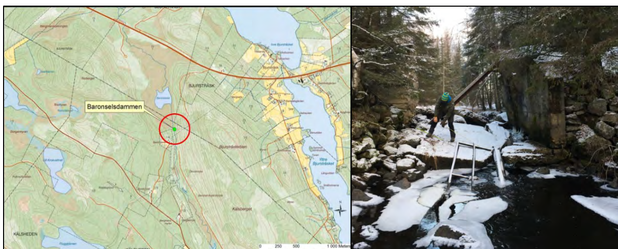
Figure 4.5. Map of the Rosån river with the Baronseldammen dam ringed and a picture of the concrete and metal debris which constitute a migration barrier for fish.
