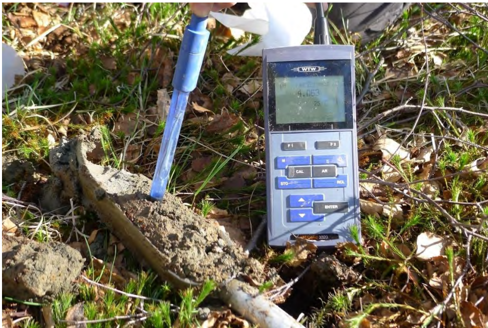
Figure 8. Measurement of pH carried out directly on the soil sample. Photograph: Gustav Sohlenius, SGU.
