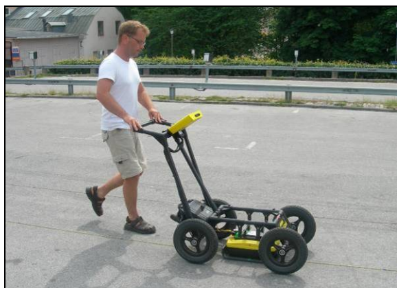
Fig. 2.2: Pär Karlsson operating the Sensors & Software Noggin Plus 500 MHz antenna mounted in the SmartCart for the survey of the upper parking place Äkroken in Nyköping. The data logger with integrated monitor is fastened in a carrier frame in front of the operator. Two profile lines with 1m separation distance are visible on the ground. The antenna is pushed along these lines and in between them with a GPR profile spacing of 25cm. Every 5cm along the profile a GPR trace is recorded.
