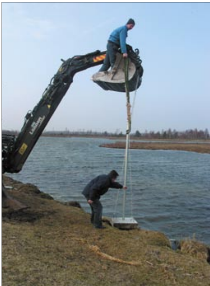
Water-level gauges were lowered into the alvarlake for monitoring fluctuations.
