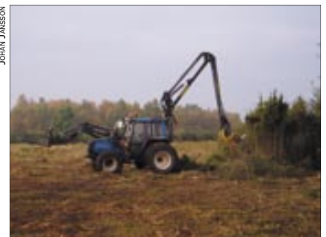
Tractor fitted with Trimcut head and a grab for piling up brushwood.
